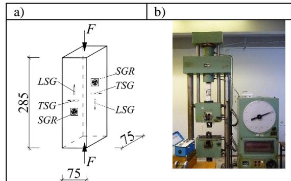
**Figure 2.** Scheme (a) and photo (b) of the compressive test
