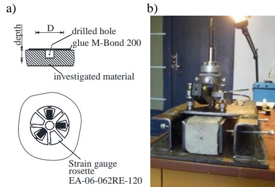
**Figure 3.** The hole-drilling technique (a) and rig for fixing a specimen (b)
