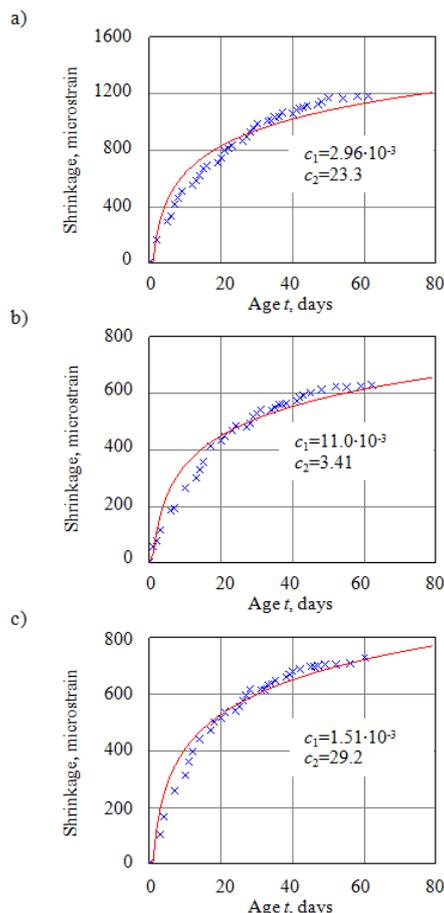
**Figure 4.** Experimental data and the curve of approximation for the specimens cast from a) MS; b) QT; c) QD
