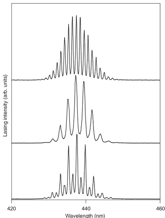
**Fig. 4.** Broadband emission spectra for three different locations of the phase step: top - double-pass spectral modulation when the step is near the back mirror; middle - single-pass modulation when the step is near the cavity center; bottom - mixed modulation when the step is near the output coupler.
