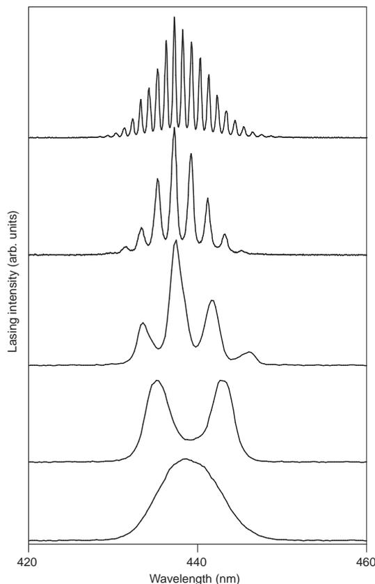
Fig. 2. Broadband emission spectra of the dye laser operated without a phase step (bottom trace) and with different phase steps (upper traces).
