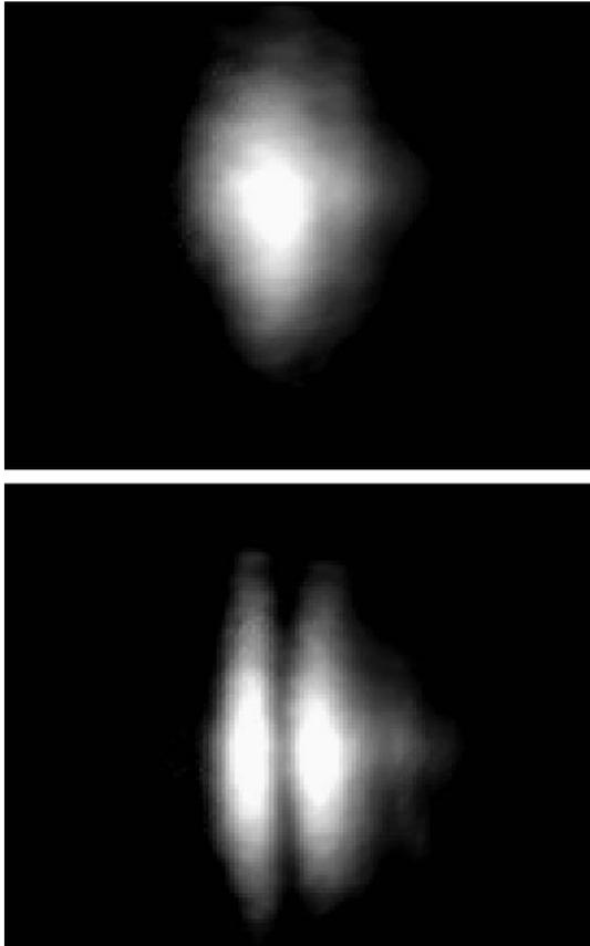
**Fig. 3.** Far-field beam profiles of the narrowband dye laser operated with an intracavity phase step: top—regular  $TEM_{00}$  mode; bottom— $TEM_{01}$ -like mode.
