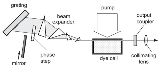
Fig. 1. Schematic view of the dye laser cavity with a phase step. For broadband lasing a plane mirror was inserted to block the grating.
