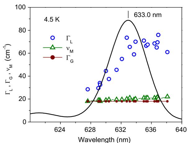
**Fig. 4.** Wavelength dependence of the spectral density function in chlorin-doped 1-propanol. The Lorentzian width,  $\Gamma_L$  (blue rings), the Gaussian width,  $\Gamma_G$  (brown dots), and the peak frequency,  $\nu_M$  (green triangles), are shown on the background of the absorption spectrum. (For interpretation of the references to color in this figure legend, the reader is referred to the web version of this article.)
