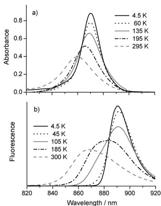
**Figure 5.** Experimental a) absorption and b) fluorescence emission spectra of LH2 complex from *Rps. acidophila* as a function of temperature.
