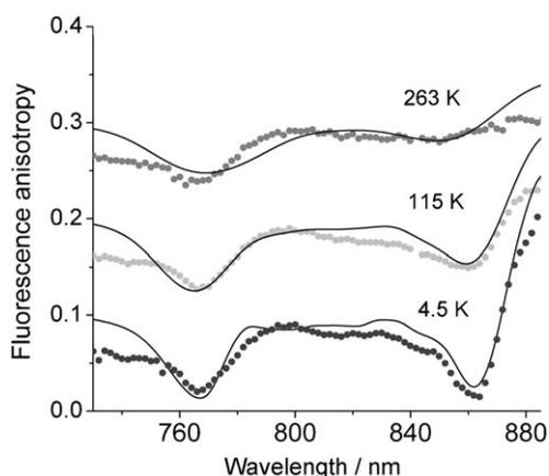
**Figure 8.** Experimental (scattered) and simulated fluorescence emission anisotropy spectra (solid lines) for LH2 complexes from *Rps. acidophila* at temperatures 4.5, 115, and 263 K. For better visibility, the middle and upper spectra are shifted vertically by 0.1 and 0.2 units, respectively.
