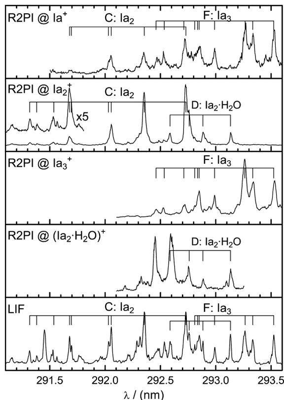
**Fig. 5.** Observed R2PI spectra detected at the mass channels of  $Ia$ ,  $Ia_2$ ,  $Ia_3$ , and  $Ia_2 \cdot H_2O$  and the (partially saturated,  $\approx 1$  mJ/pulse, off-axis pumped) LIF excitation spectrum from Fig. 4 for comparison. All R2PI spectra are measured with  $\approx 0.1$  mJ ionization laser pulses without water addition.
