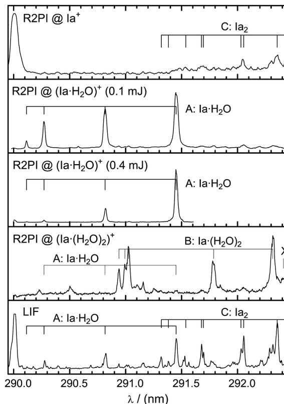
**Fig. 6.** Observed R2PI spectra detected at the mass channels of Ia, Ia·H<sub>2</sub>O, and Ia·(H<sub>2</sub>O)<sub>2</sub> and the (partially saturated,  $\approx 1$  mJ/pulse, off-axis pumped) LIF excitation spectrum from Fig. 4 for comparison. All R2PI spectra measured with  $\approx 0.1$  mJ ionization laser pulses (0.4 mJ in the third panel) without water addition, except for the Ia·(H<sub>2</sub>O)<sub>2</sub> R2PI spectrum measured with addition of water.
