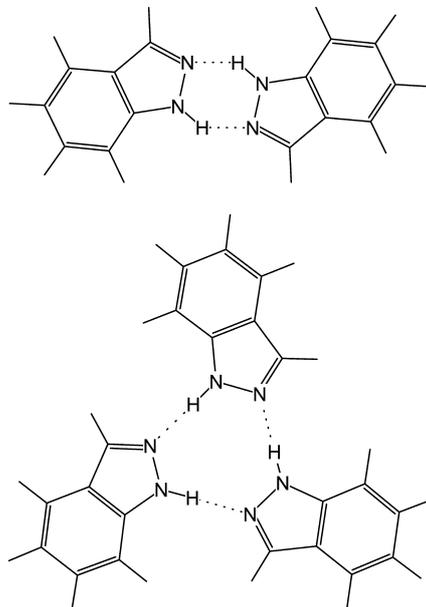
**Fig. 1.** Symmetric planar hydrogen-bonded structures of the indazole ( $\equiv$ benzopyrazole) dimer (Ia<sub>2</sub>) and trimer (Ia<sub>3</sub>) proposed by analogy with the *ab initio*-predicted structures of the dimer and trimer of pyrazole [10, 11].
