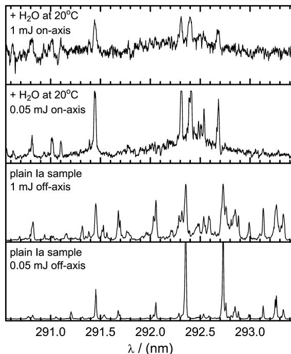
**Fig. 4.** Effect of optical saturation and water addition on the LIF excitation spectra under different experimental conditions. The zero of the vertical scales for all spectra corresponds to the zero-level of the signal intensity.
