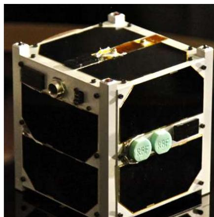
Figure 1 ESTCube-1 satellite before delivering it to the launch provider.
