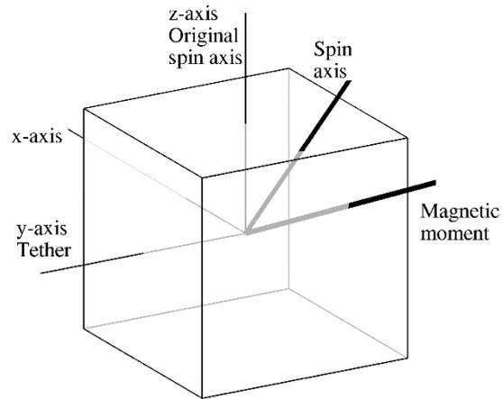
*Figure 3 Alignment of the spin axis under stable unactuated conditions as well as the originally intended spin axis (aligned with z-axis), the tether (aligned with y-axis) and the magnetic moment under unactuated conditions.*
