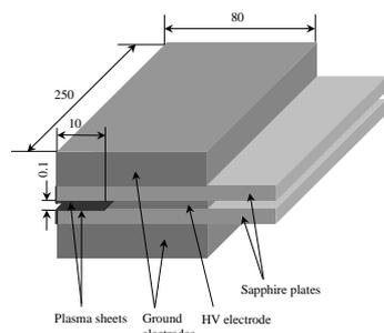
**Figure 1.** Schematic of the sliding discharge electrodes. Spontaneous emission from two arc-free plasma sheets (250x10x0.03 mm) is measured in the direction of the long axis.
