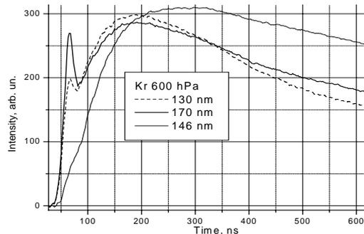
**Figure 7.** Time-resolved emission of the first (130, 170 nm) and the second (146 nm)  $\text{Kr}_2$  continua at gas pressure of 600 hPa.
