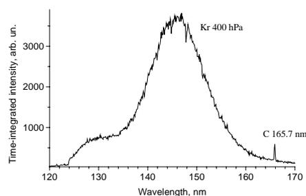
**Figure 2.** Time-integrated emission spectrum of a sliding discharge at a Kr pressure of 400 hPa.
