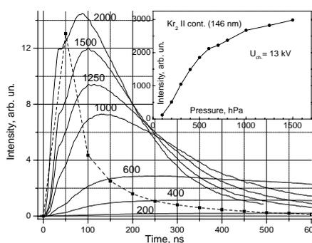
**Figure 4.** Time-resolved emission intensity of the second  $\text{Kr}_2$  continuum (146 nm) in sliding discharge at different pressures (hPa). Dashed line is a time behavior of  $\text{Kr}^*$  587 nm emission line, measured at 1250 hPa. The inset shows time-integrated intensity of the second  $\text{Kr}_2$  continuum at different pressures at a fixed charging voltage (13 kV).
