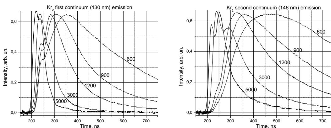
**Figure 5.** Time-resolved emission (normalized intensity) of the first (130 nm) and the second (146 nm) Kr<sub>2</sub> continua at different gas pressures (hPa). Discharge pumping pulse (FWHM) is about 20 ns.
