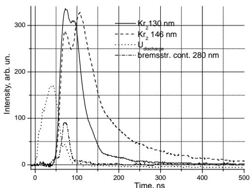
**Figure 6.** Time behaviors of the discharge voltage,  $\text{Kr}_2$  the first (130 nm), the second (146 nm) and bremsstrahlung (280 nm) continua at pressure of 5000 hPa.
