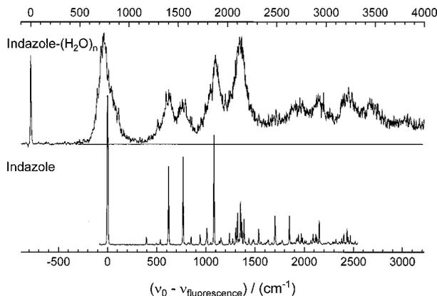
FIG. 7. The DF spectrum of indazole–water complexes showing strongly broadened ( $\approx 150 \text{ cm}^{-1}$ ) spectral features. The spectrum was observed after excitation of a weak  $S_1$  band at  $324 \text{ cm}^{-1}$  blue from the electronic origin of the free indazole monomer (upper trace). The  $S_1$  origin DF spectrum of the monomer is shown for a comparison in the lower trace.
