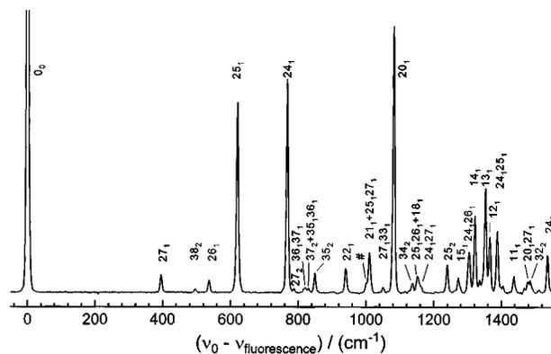
FIG. 5. The measured DF spectrum of indazole following excitation of the  $S_1 \leftarrow S_0$  ( $0_0^0$ ) origin (resolution:  $\approx 7 \text{ cm}^{-1}$ ). The # marks an unassigned band at  $1000 \text{ cm}^{-1}$ .
